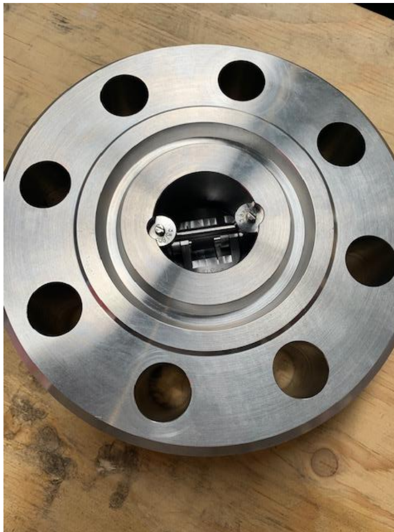
2" class 1500 Dual plate check valve
