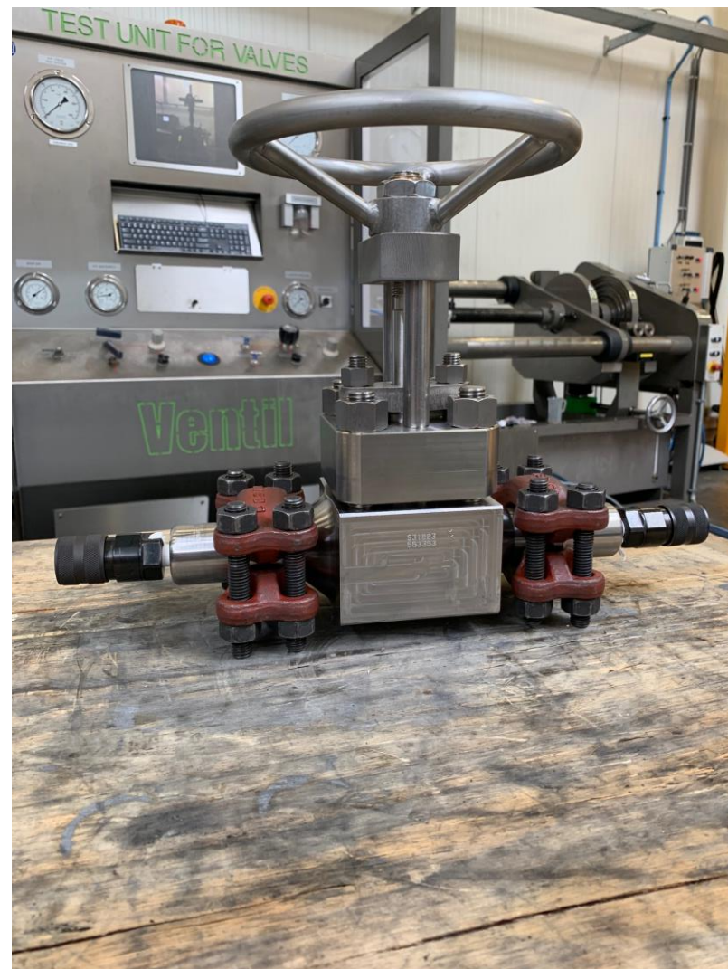
2" class 2500 Gate Valve special hub ends
