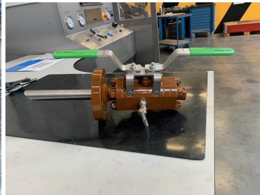
2" class 300, needle valves, quill design
