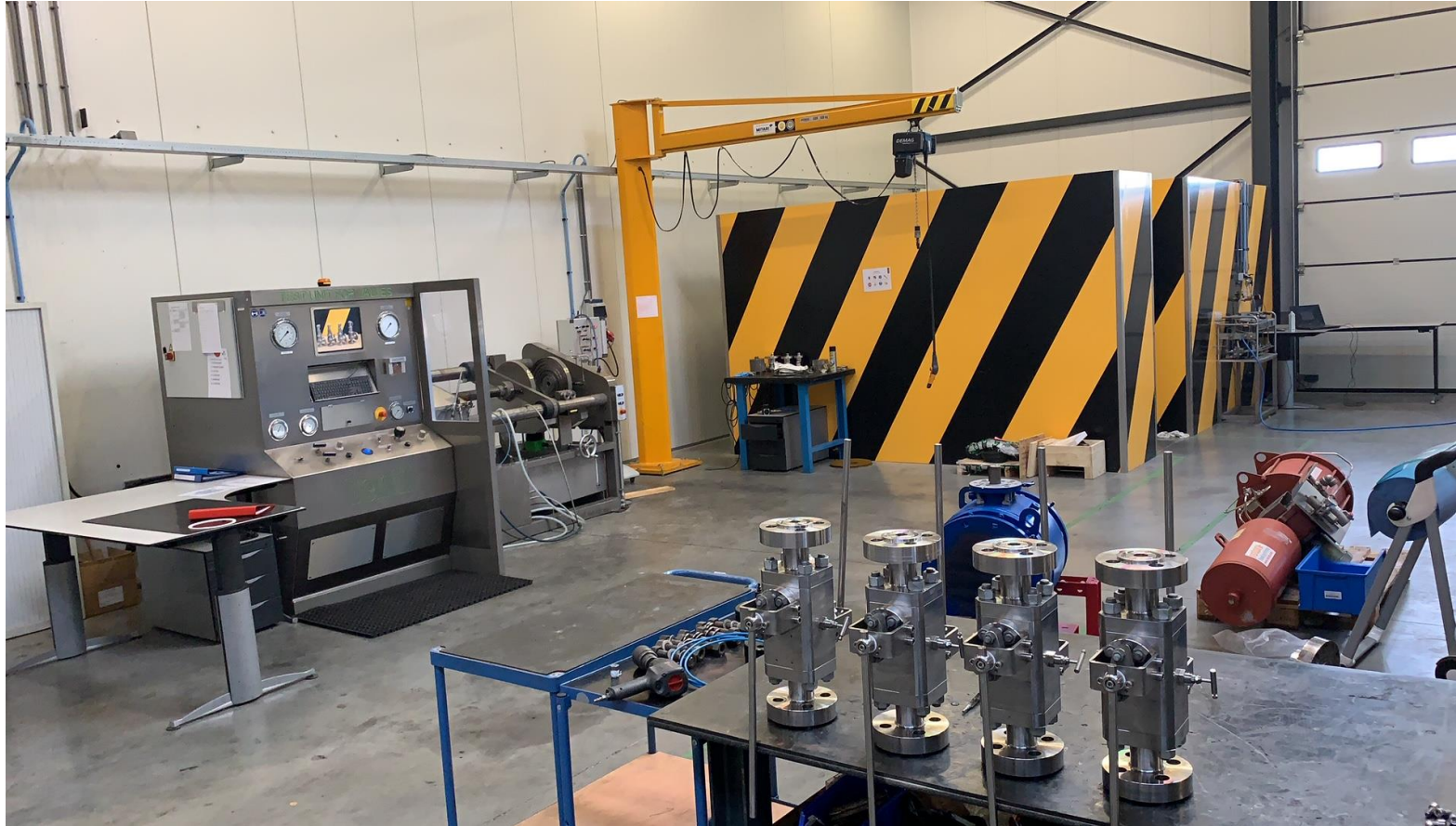
High Pressure Gas booster up to 2150 bar
