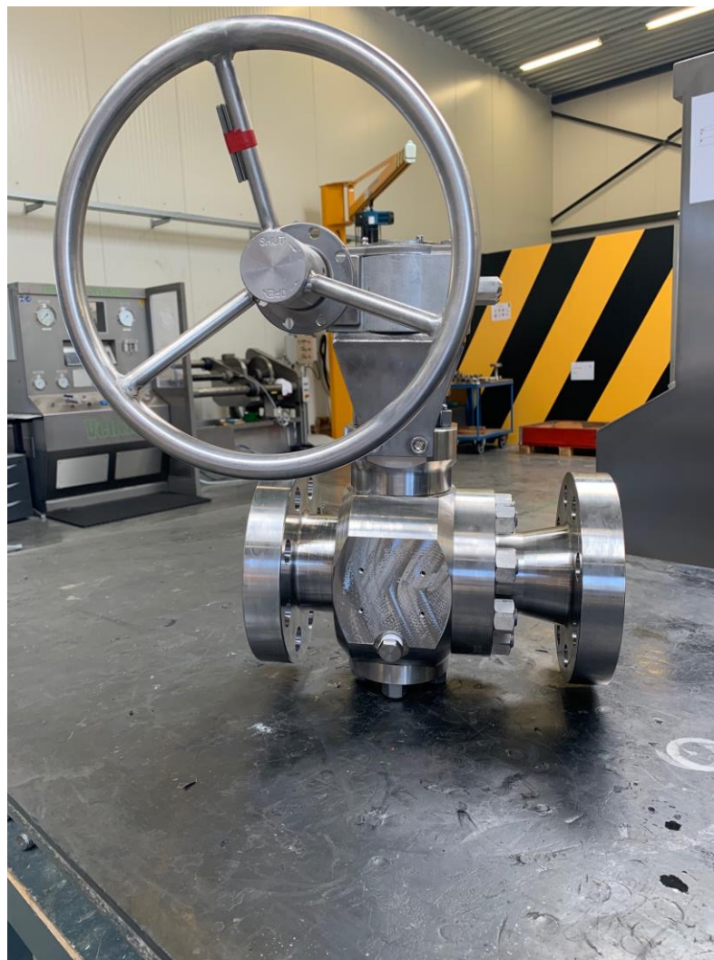
3" class 1500 side entry ball valve
